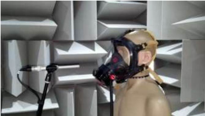
Figure 7. 無響室でSCBAを装着したGRAS社製KEMARマネキン [Photo courtesy of Scott Safety, used by permission.]
